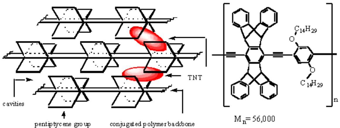
Figure 2, the intercalation of TNT in the receptor and the structure of the receptor molecule
