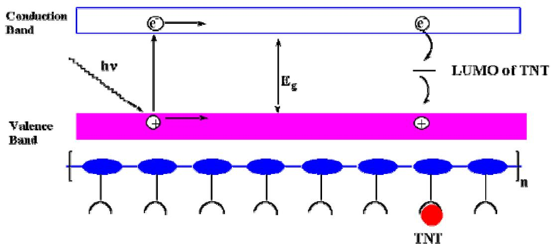
Figure 3 – How TNT changes the fluorescence properties of the polymer
